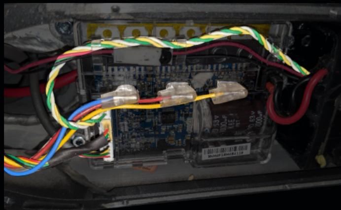
Remove the controller by first unscrewing the retaining screws.
